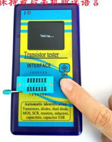
1. Install the 9V battery and press the TEST button.
